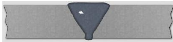
Figure (II.19): types d'inclusions solides.
