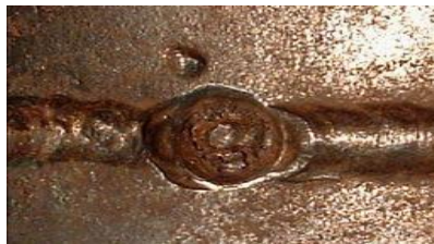
Figure (II.26): Effondrement.
