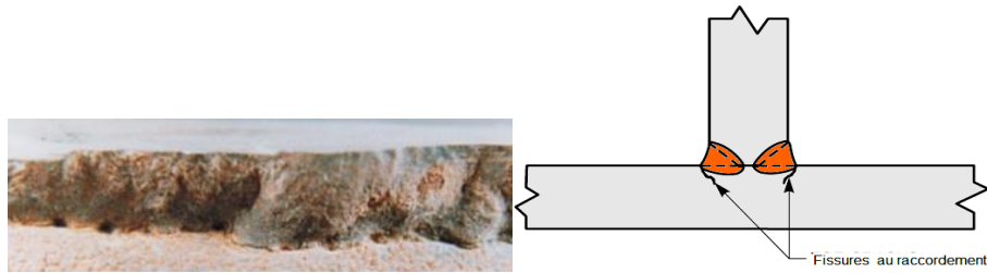
Figure (II.5) : Fissures au raccordement.
