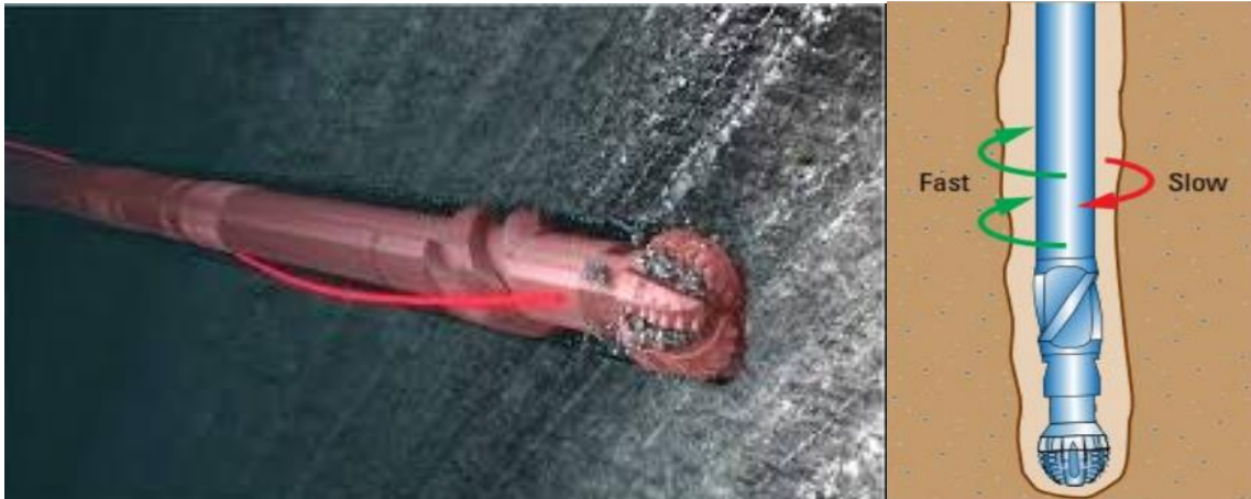
Figure 2-4 Vibration torsionnelle ( Stick-Slip )
