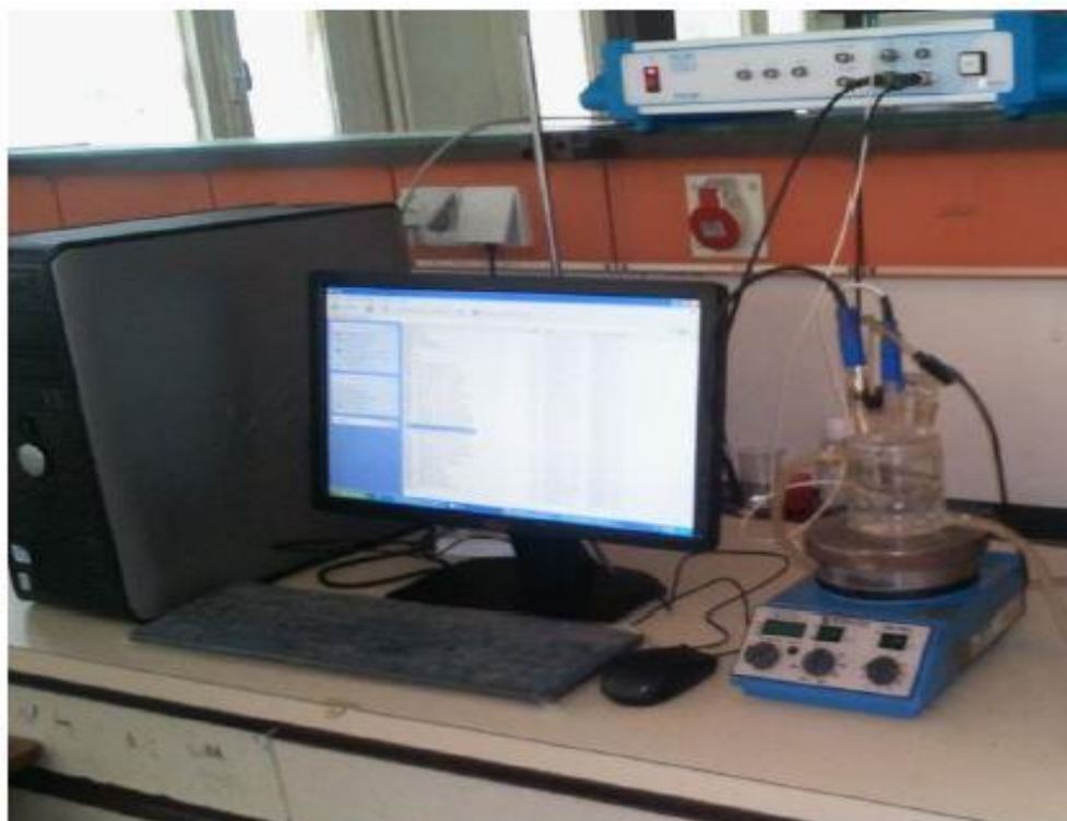
Figure II. 1: Schematic representation of the experimental device used for the elaboration of ZnS nanostructures.
