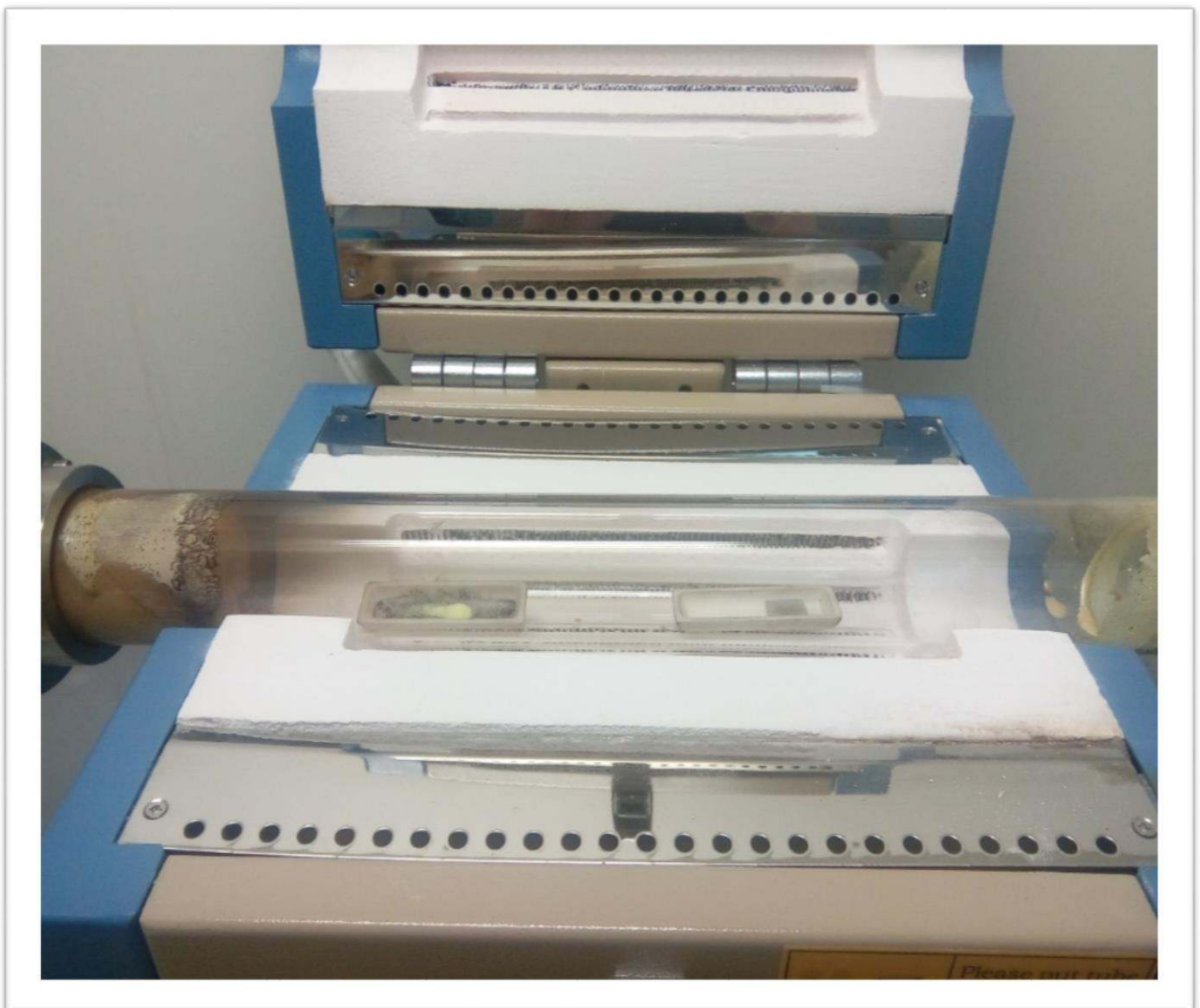
Figure III. 28 : Tube furnace for annealing under a sulfurized atmosphere
