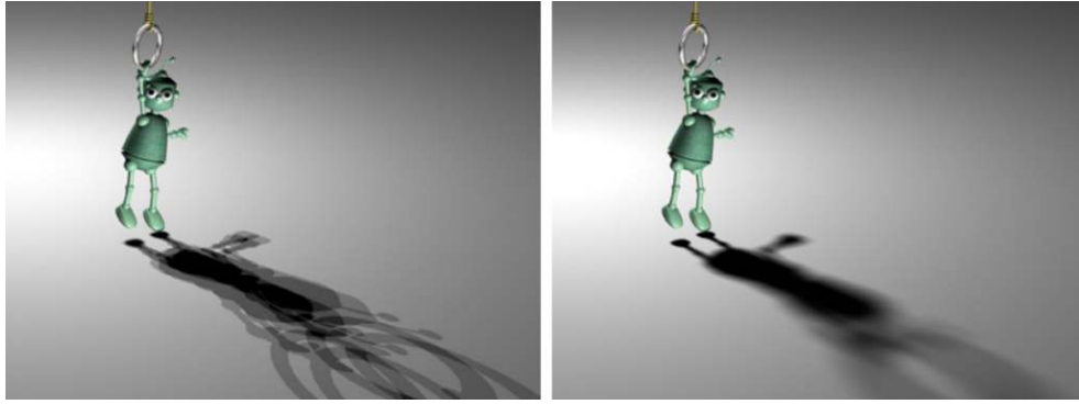
Figure. 2.17. Comparing two images rendered with different samples of the area light source. Left image: soft shadow computed using 4 samples. Right image: soft shadow computed using 1024 samples [HLHS03].
