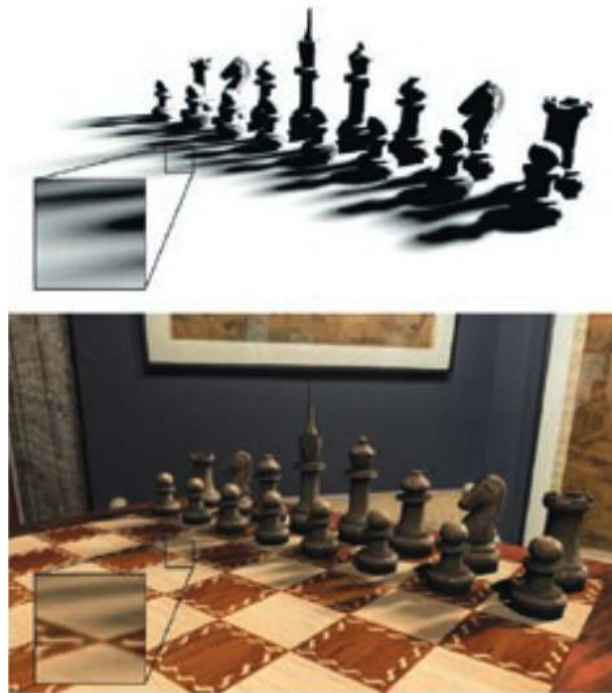
Figure. 1.13. Naive ray-traced shadows using 256 samples per pixel running at 200 ms per frame. Times measured using a GeForce RTX 2080 Ti GPU. Top: visibility buffer. Bottom: final image [BWB19].
