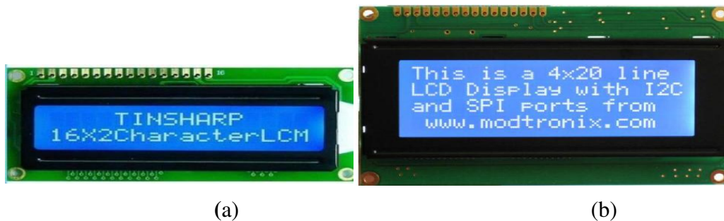
Figure 2.9 : Afficheurs LCD (a) (16x2) (b) (20x4)
